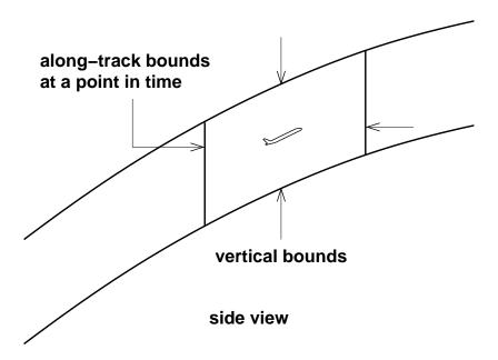
Figure 2: Trajectory bounds in the longitudinal plane
